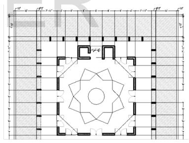
Fig6. The main prayer hall plan with detail dimensions
